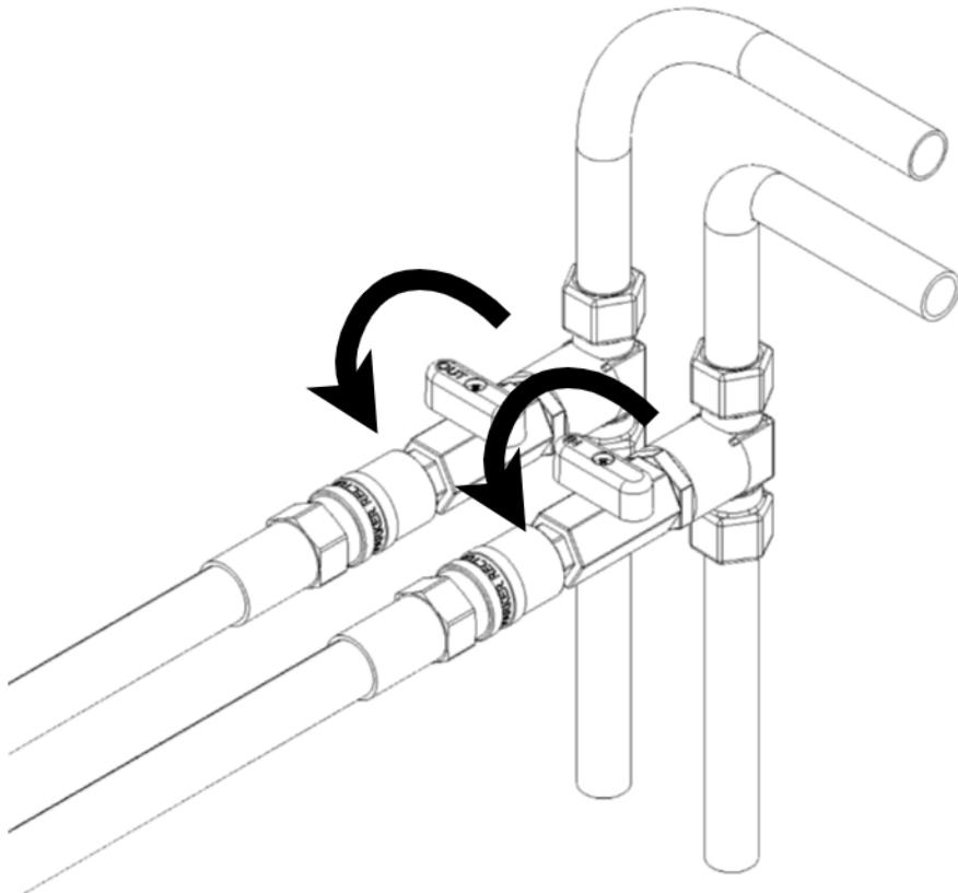
5. After reconnecting the Chill, make sure that the pressure level in your heating system is satisfactory (between 1 and 2 bars). If the pressure is too low, refill it by using the filling valve close to your boiler or below your HeatCharger.
