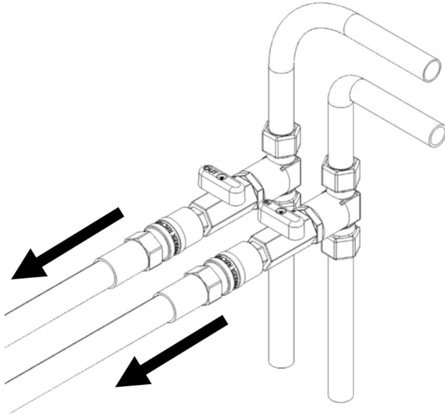
3. Do not disconnect the pipes from the Chill device. The water inside the unit will be contained and the Chill will be ready to operate after being reconnected to the other set of connectors.
